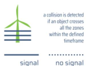
The basic principle of B-finder is the sequence of recordings of animal falling across the sensor zones. The fall of dead or injured animals has different parameters than the flight of those alive. B-finder system differentiates between them and reports only the fatalities. The monitoring results are available online for the user including information about the time of collision and the location of the carcass.
