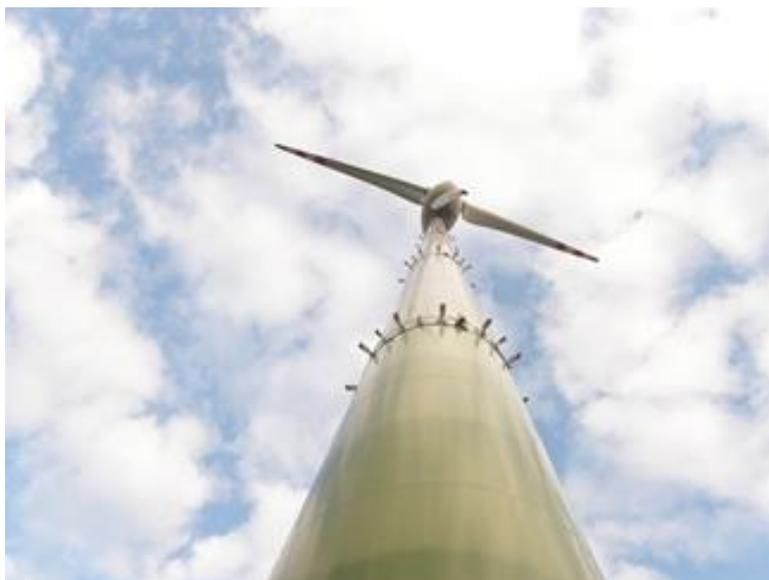
Figure 1. B-finder prototype sensors on the wind turbine.
