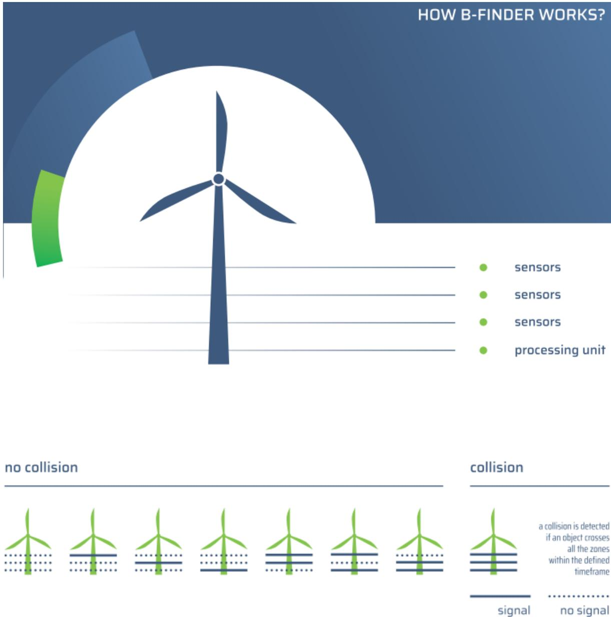
The basic principle of B-finder is the sequence of recordings of animal falling across the sensor zones. The fall of dead or injured animals has different parameters than the flight of those alive. B-finder system differentiates between them and reports only the fatalities. The monitoring results are available online for the user including information about the time of collision and the location of the carcass.
