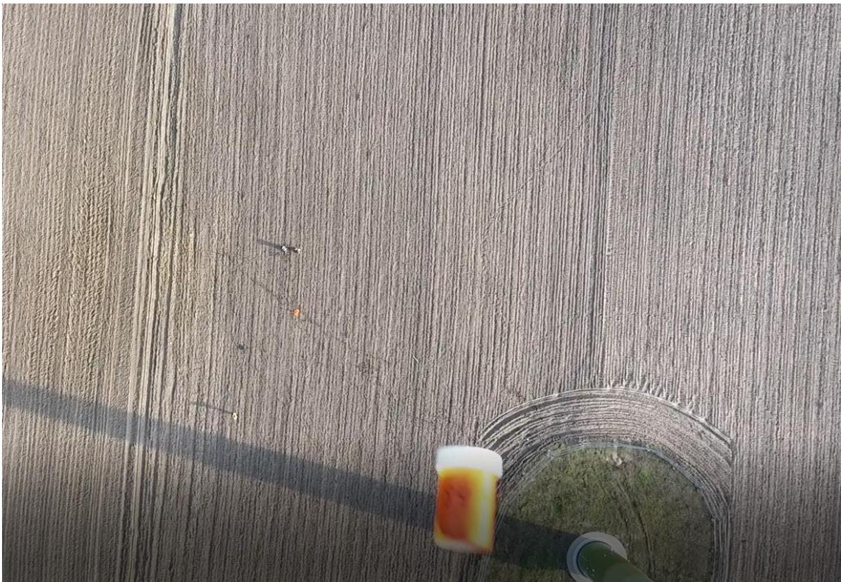
Figure 15. A test tube falling down after being dropped by the drone. Its flight is recorded not only by the prototype but also by the camera attached to the drone.
