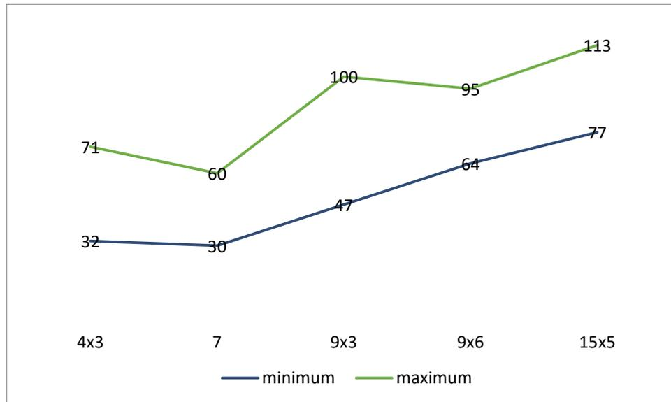
Figure 17. The minimum (in the worse conditions) and maximum (in the best conditions) detection range [m] for objects of different size [cm].
