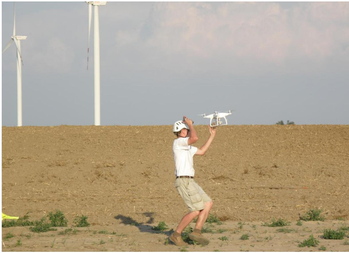
Figure 12. Loading a test tube onto the drone. The technician holds in his right hand a pyrometer, which is used to measure the temperature of the object just before the loading and immediately after the fall.
