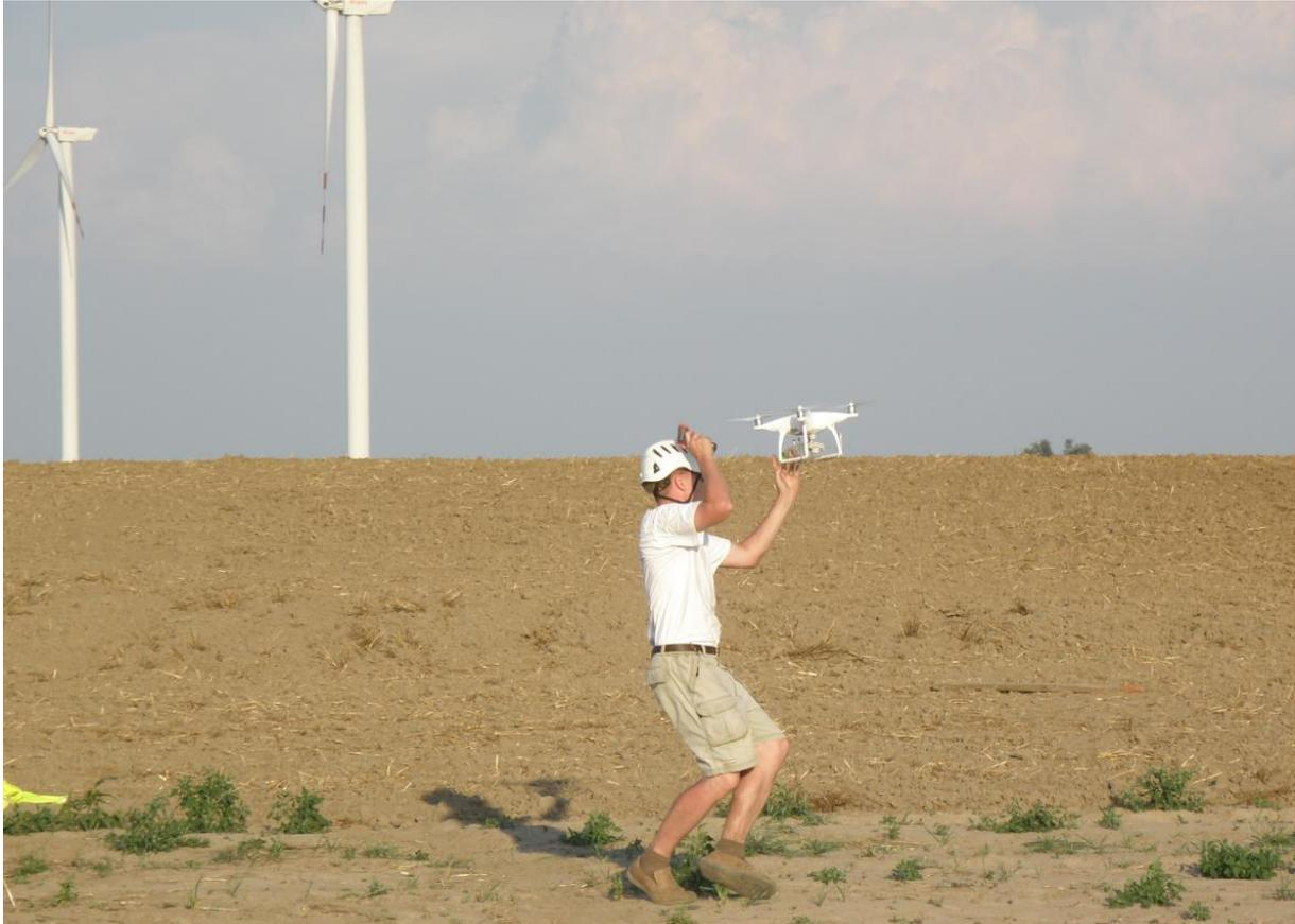
Figure 12. Loading a test tube onto the drone. The technician holds in his right hand a pyrometer, which is used to measure the temperature of the object just before the loading and immediately after the fall.
