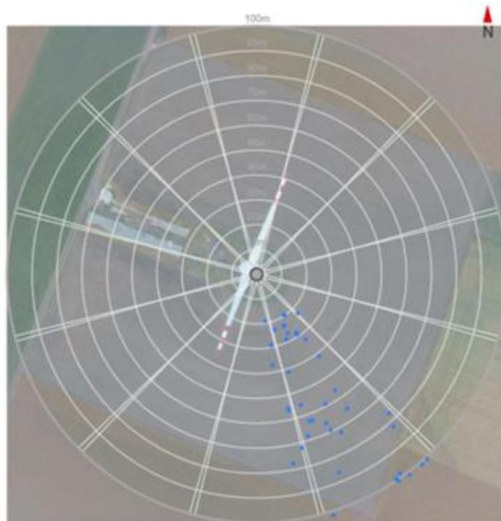
Figure 16. Locations of the dropped objects estimated by the B-finder system, shown in the user panel (tests on 2018.08.17). The automatic results were compared to manual measurements.
